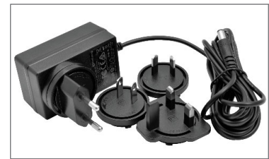
Universal power supply included 24 VDC/1 A - 100÷240 VAC input 3 m cable length
