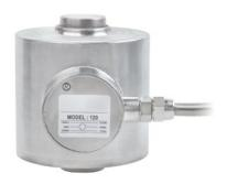
The Model 120 has a stainless steel housing to protect against corrosion. The alloy steel compression element is nickel-plated, and the rocker mounting accessories are zinc-plated alloy steel.
