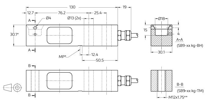
For maximum capacity from 250kg to 1,000kg: Mounting bolts M12 8.8; torque 90Nm For maximum capacity of 2,000kg: Mounting bolts M12 10.9; torque 120 Nm Torque values assume oiled thread.
