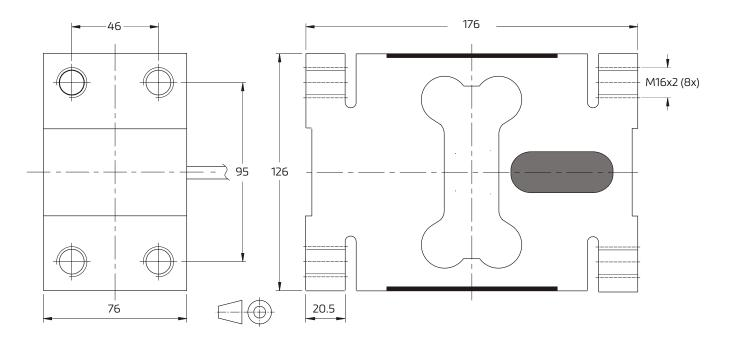
Mounting bolts M16x2; torque 200 Nm. Torque value assumes oiled threads.
